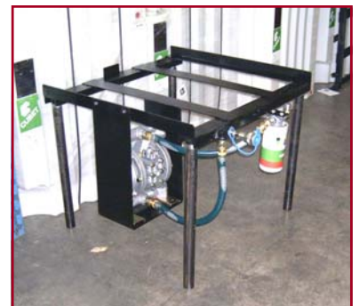
SDS Stand with Diaphragm Pump Installed
