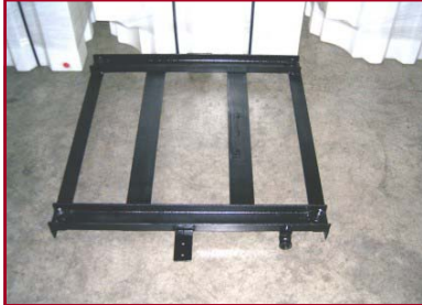
(Fig.2) Stand Base with pump hanger installed
